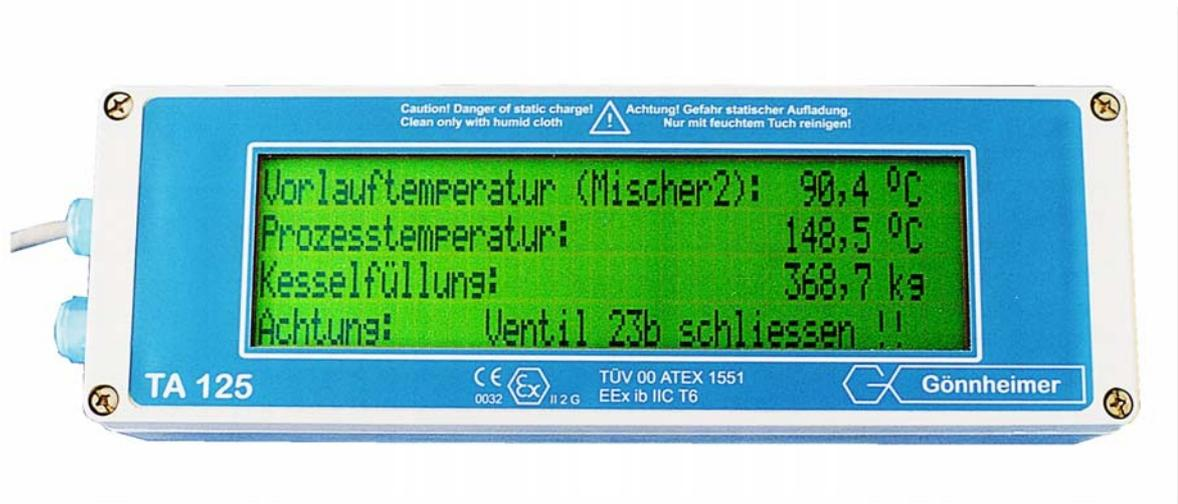
The TA125 stores up to 32 kByte of messages in an internal EEPROM. You can program the stored messages with the bundled windows software "TEXT LINK". There are two ways to display the stored texts: the serial interface or applying a defined bit pattern to binary address inputs of the TA125 (option).
